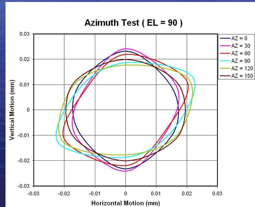
**Measured Distortion of cell as Telescope moves in Azimuth**
